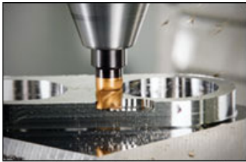
Applying the replaceable-tip concept to milling cutters like the CoroMill 316 follows from the fact that solid-carbide tools typically take less than 1xD depth of cut, so all that expensive carbide flute length isn't needed.
