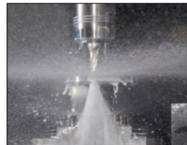
Replaceable-tip drills like the Qwik-Twist line address the number of drills that are typically "in-float" when using solid-carbide tools. Photo courtesy Ingersoll Cutting Tools
